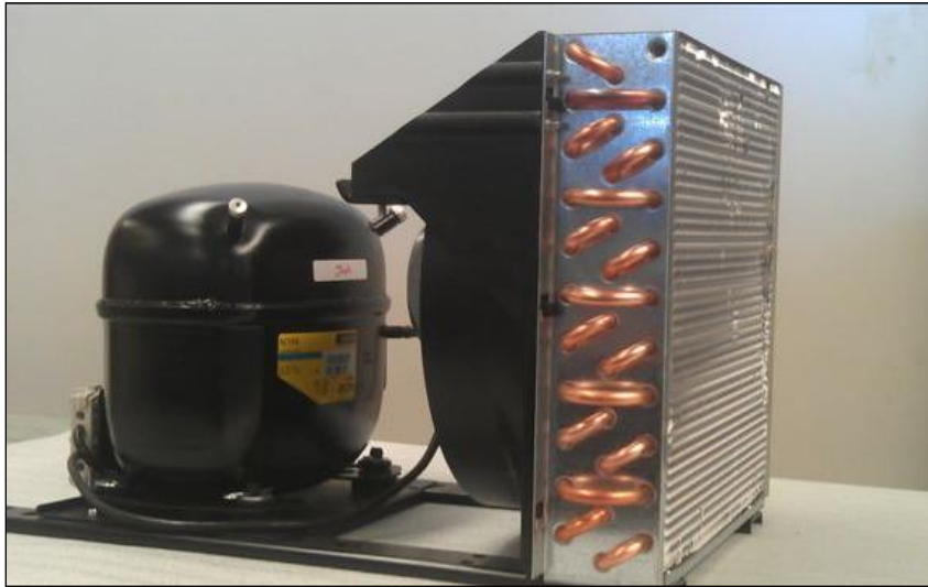
Remote condenser unit
